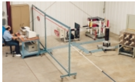
IN HOUSE 200KV IMPULSE GENERATOR TO TEST BIL WITHSTAND
