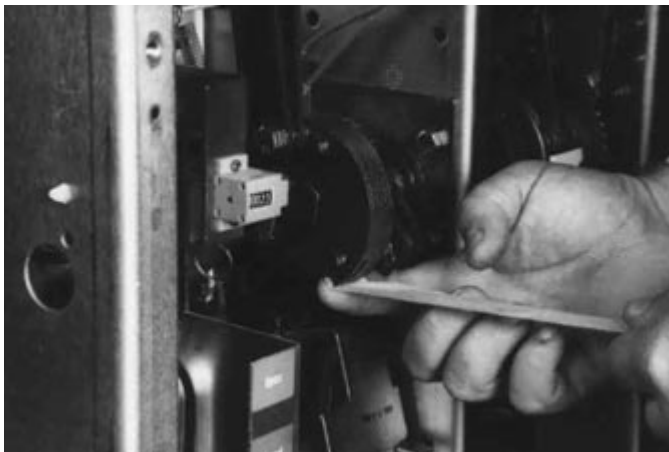
Figure 6-6 Starting Tape at Bottom of Cam
