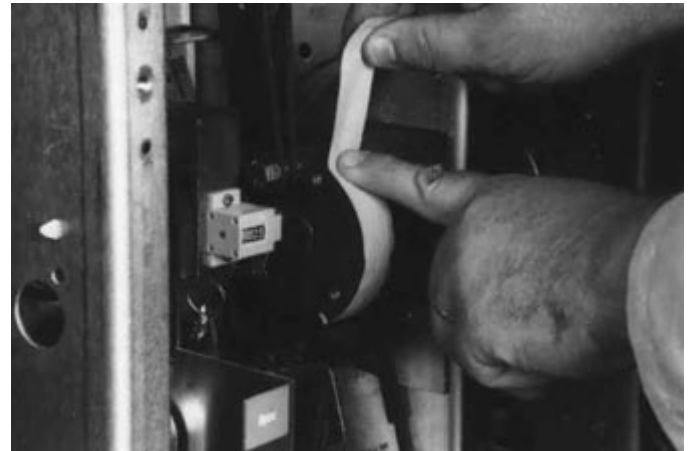
Figure 6-7 Wrapping Tape Up Around Cam
